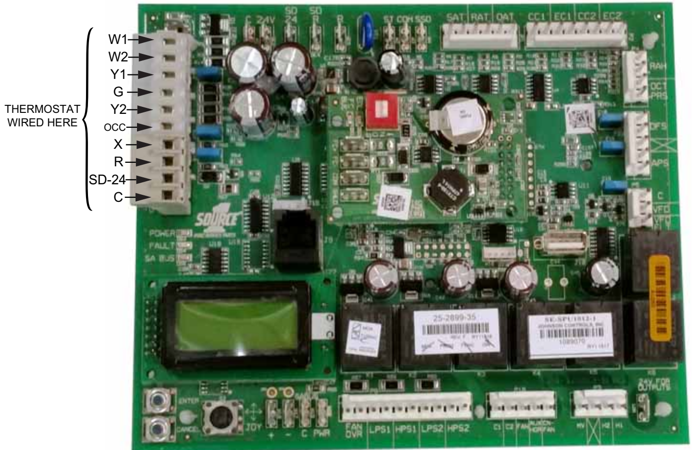
Figure 24: Unit Control Board
